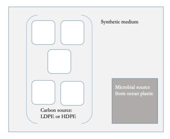
**Figure 1.** Microcosm setup. PE pieces previously incubated in the ocean were used as source of microbes. The synthetic medium imitated ocean salinity but contained no carbon source. Carbon was provided as sterilized PE fragments (5 per culture).
