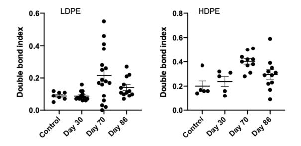
**Figure 5.** Double bond index values calculated from the samples of the three microcosm experiments using FTIR.
