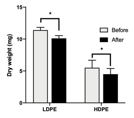
**Figure 3.** Average dry weight significantly decreased for both LDPE (M=11.4 mg, SD=1.35 to M=10.1 mg, SD=1.37) and HDPE M=5.5 mg, SD= 2.89 to M=4.5 mg, SD= 2.17) after the micro-cosm incubation. As controls PE fragments sterilized and UV-treated but not incubated were used. The \* indicates significant differences of p=.0133 and p=.0409 for LDPE and HDPE, respectively.
