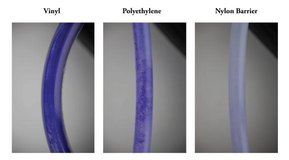
**Figure 1. Crystal violet staining of draught lines.** Following a sixteen-week simulation, each draught line was drained, rinsed with DI water, and stained with crystal violet. Qualitative images were taken to compare relative biofouling.
