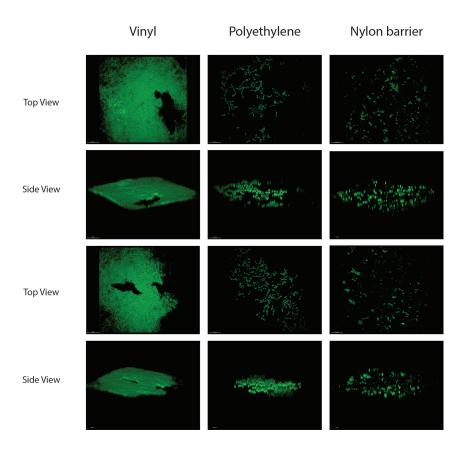
**Fig. 3. Confocal imaging of adhered biofilm.** Six 25 mm segments were taken from each draughtline, stained with a fluorescent dye, and observed on a confocal microscope with an excitation wavelength of 480 nm and a 63x oil immersion objective.
