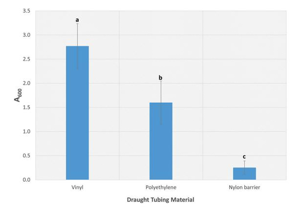
Figure 2. Quantifying biofouling of draught lines. Six 25 mm segments were taken from each draught line and stained with crystal violet. The stained biofilm was solubilized with DMSO, transferred to acuvette, and absorbance was measured at  $\lambda 600$ . Errorbarsrepresentstandarddeviation in each group. Significant differences wereobtained between groups indicated with different letters;
