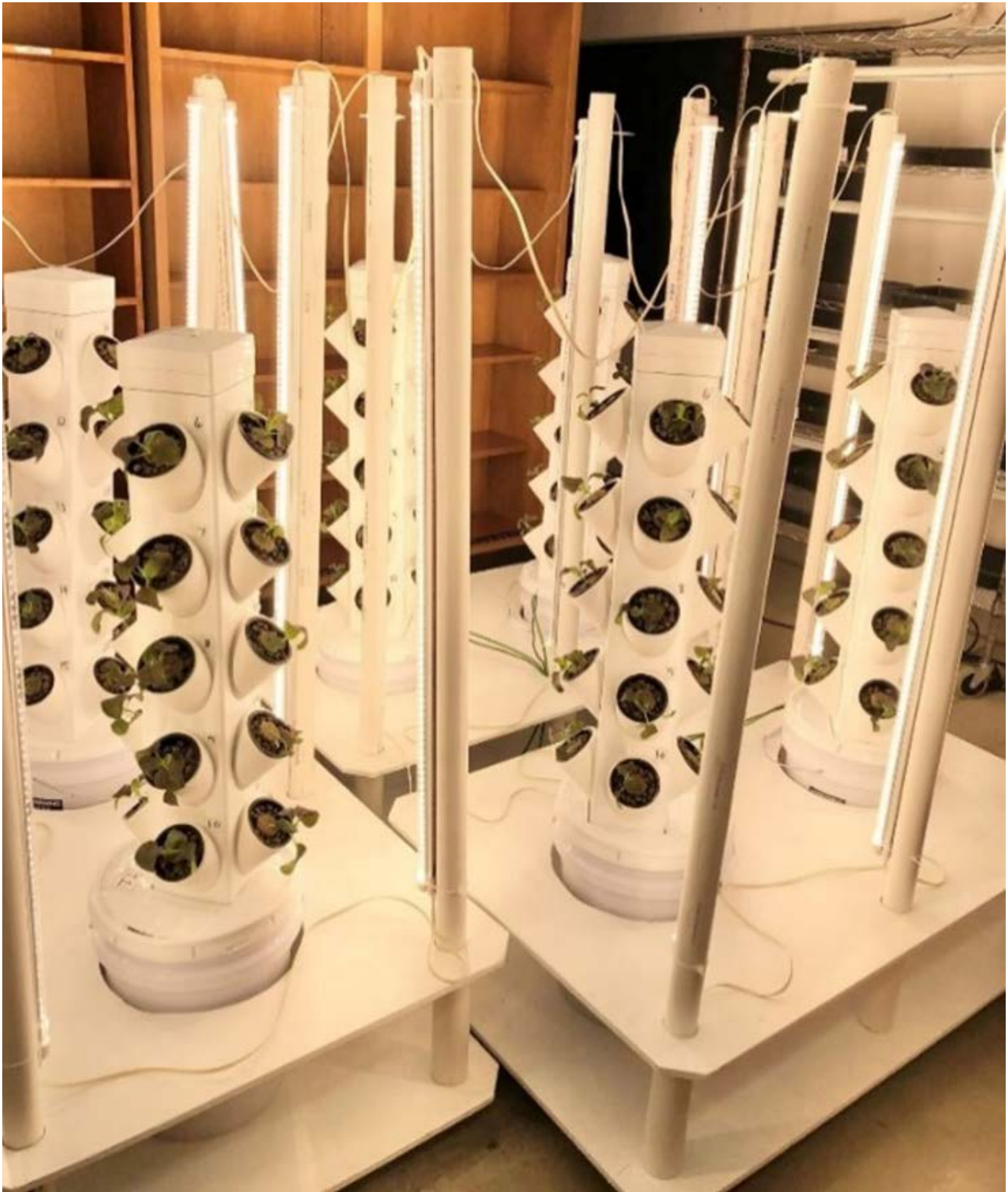
Fig 1: Design layout of the three modular units which housed the six vertical grow towers that were surrounded by six strips of LEDs each. The photo was taken in Weston Hall, room 1208, at Northern Michigan University, in Marquette, Michigan, where the experiment was conducted from September 2020 - March 2021.
